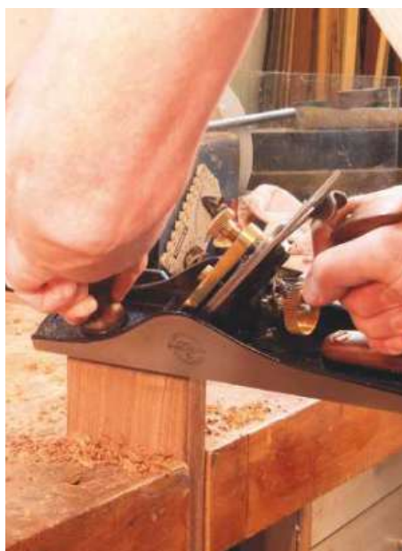
▲ Pic.4 Planing the outside of the knuckle using the new Rider series No.5
